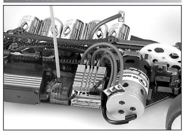
The speed controller must be placed in a cool and crash-protected area in the car.
